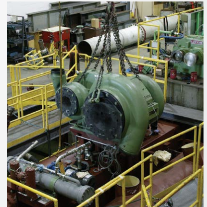
Multi-stage carbon monoxide compressor being prepared for closed-loop testing
