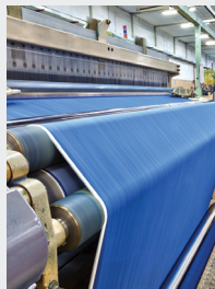
Textile High-tech air jet looms require super clean 100% oil-free air
