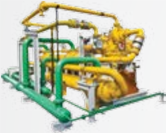
The three-stage MSG-3 compressor pictured above boosts the pressure of natural gas entering power generation turbines at a combined cycle power plant in Russia
