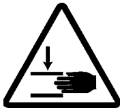
Pinch point hazard. Keep hands clear.
